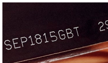
Laser mark on coated cardboard box
